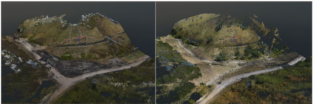
LiDAR images of the Horizon Mine in Utah, before and after reclamation
