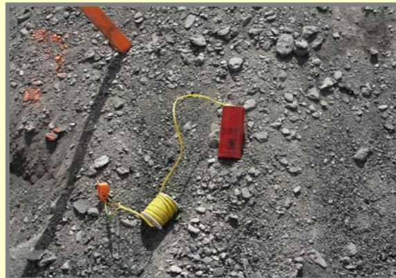
Photograph showing 1-pound cast primer with electronic detonator.
