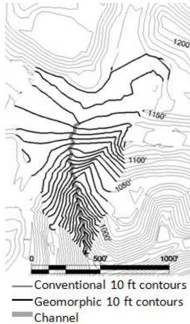
Figure 17. Geomorphic design for VF2 in permitted area with maximum fill volume (Design 10).
