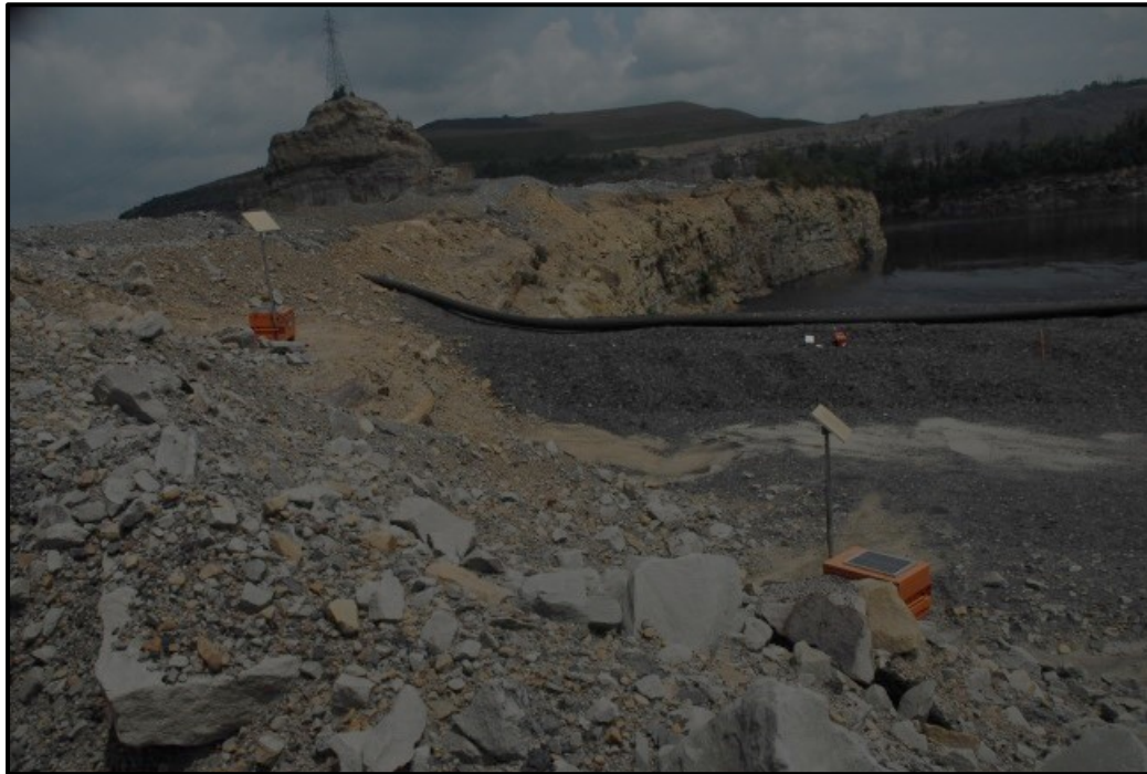
Figure 32 Showing Company Seismograph 1 on Dam (on right) and Company Seismograph 2 on Solid Bank (on left)
