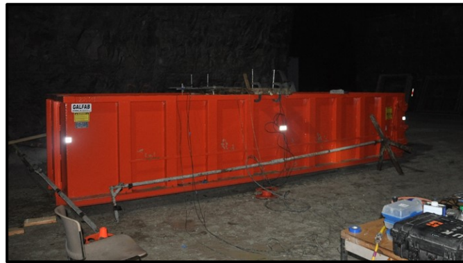
Figure 11 Galfab gasketed open top container where tests were performed. (Larson-Robl et al. 2015)
