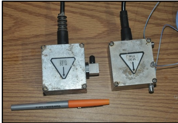
Figure 13 Left: seismograph unit 5595 with a triaxial accelerometer, Right: seismograph unit 1746 with uniaxial accelerometers in each component. (Larson-Robl et al. 2015)
