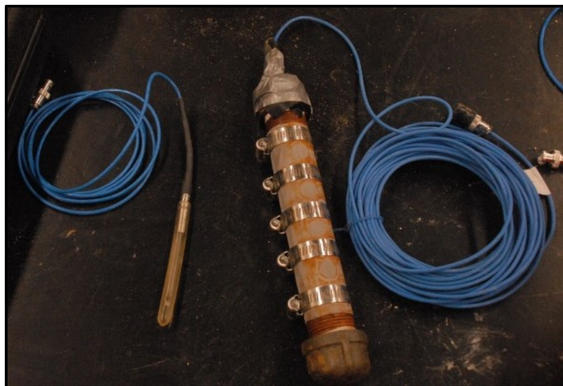
Figure 26 Tourmaline sensor without (on left) and with (on right) screening device
