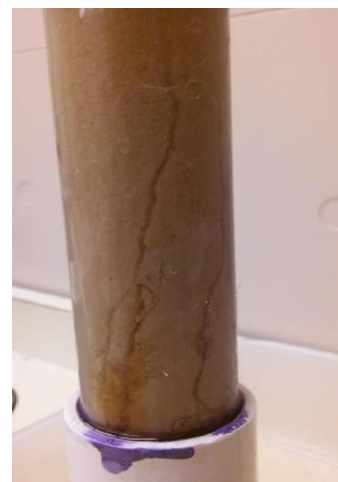
Figure T5.12 channelization in filter media
