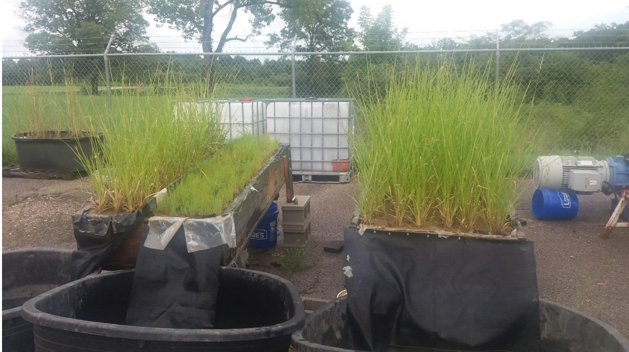
Figure T3.7 Task 3 set up with sediment check containers (dams) at week 12
