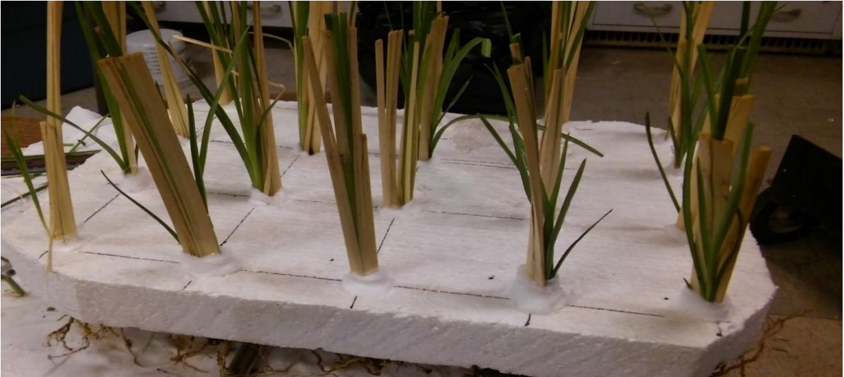
Figure T6.2 Vetiver floating platform for field study of AMD hydroponic treatment
