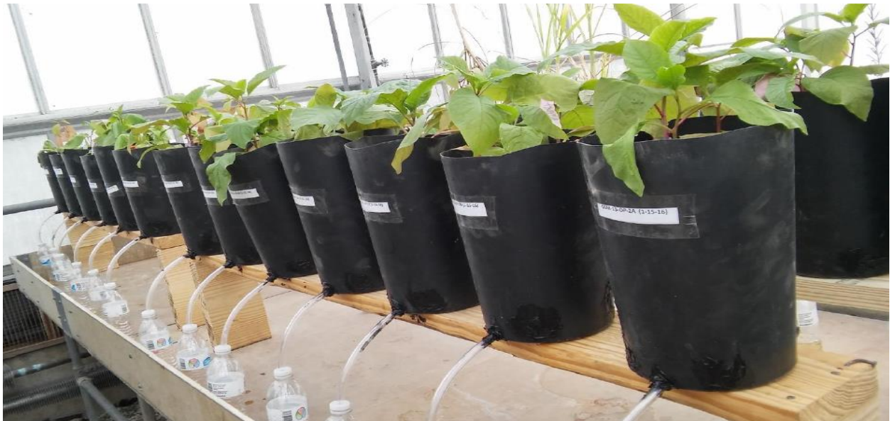
Figure T2.13 Column study experimental setup (Pokeweed) at SIU's green house facility
