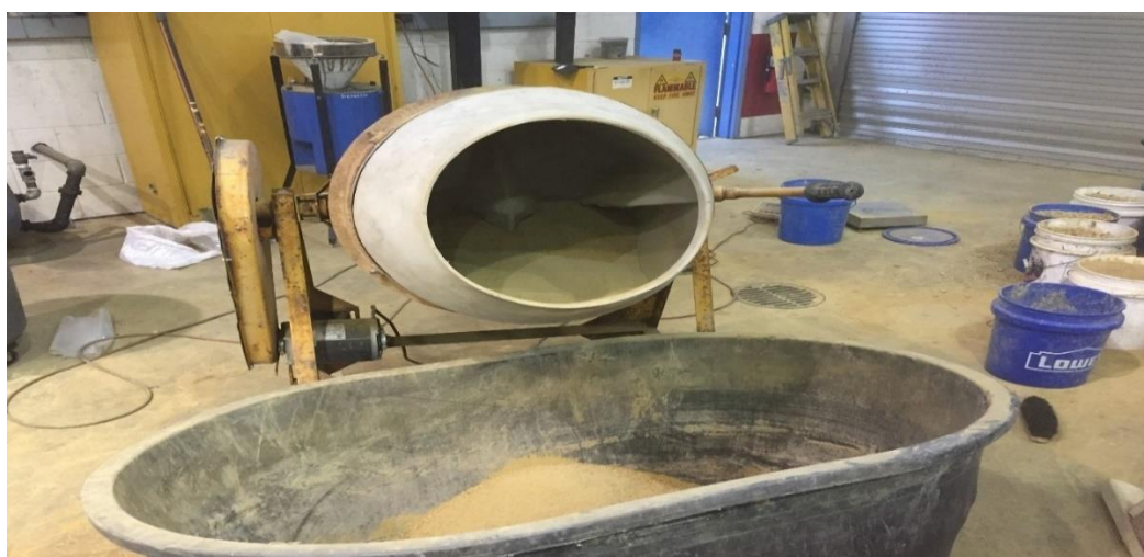
Figure T3.2 Preparation for incubation test –mixing of WTR with AMD impacted soil.
