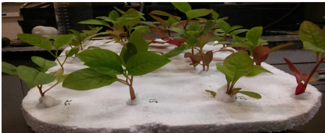
Figure T6.1 Pokeweed floating platform for field study of AMD hydroponic treatment
