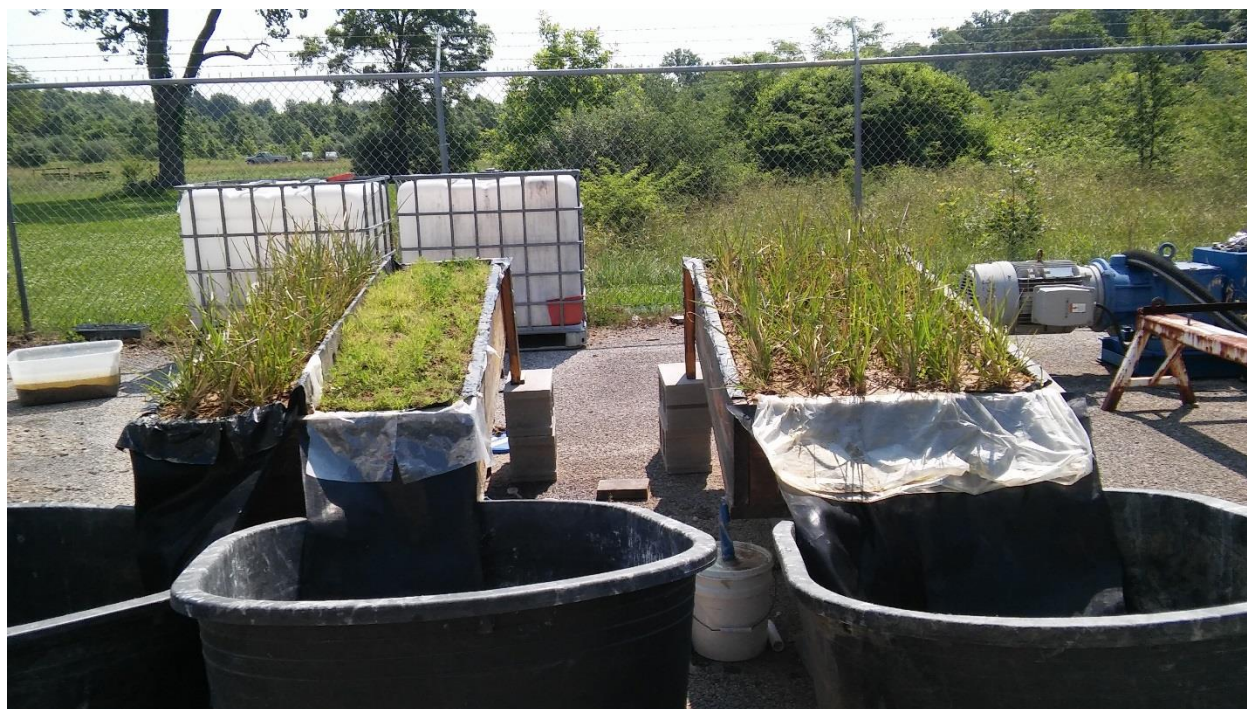
Figure T3.6 Task 3 set up with sediment check containers (dams) at week 2
