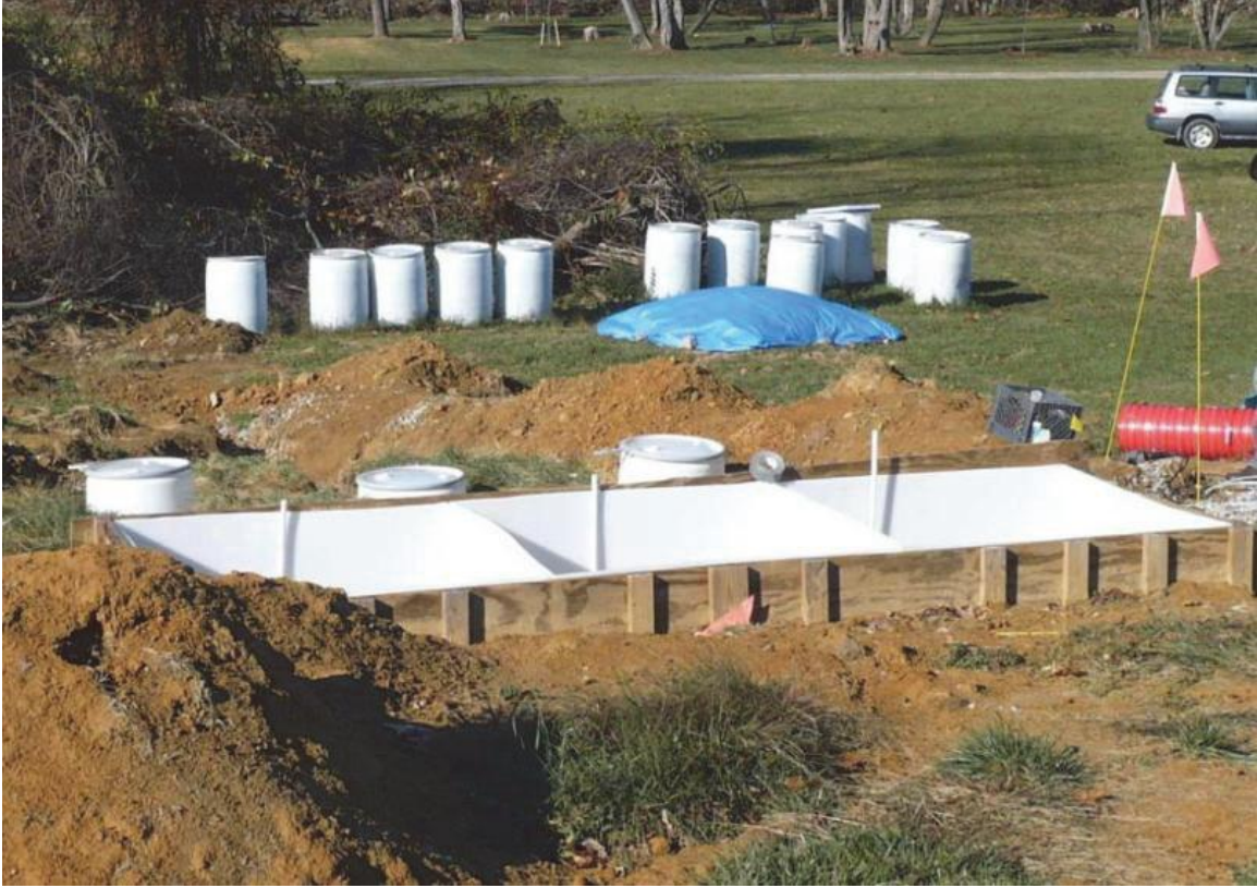
Mesocosm prior to filling with Harlan sandstone spoil.
