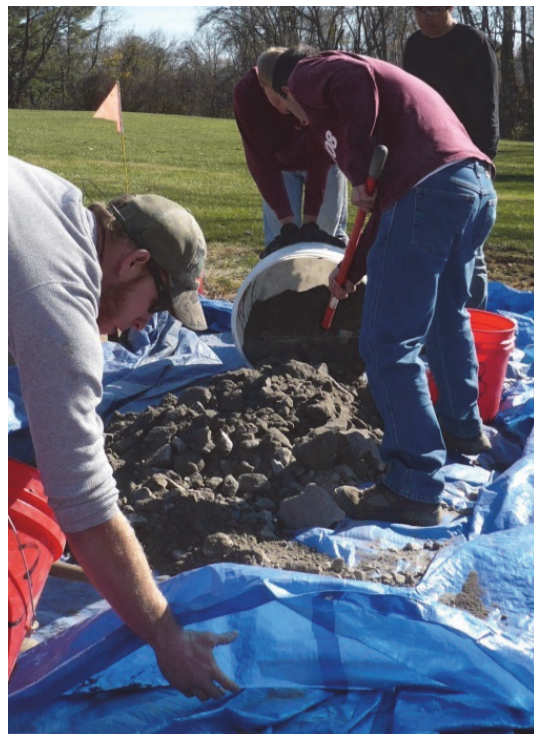
Figure 3.4. Homogenizing Harlan sandstone spoil prior to placement in mesocosms and barrels.
