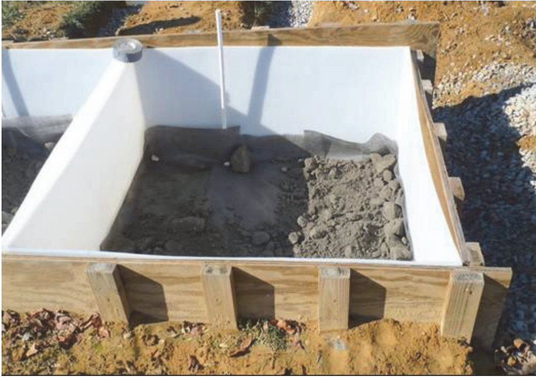
Figure 3.5. Initial placement of Harlan sandstone spoil over landscape fabric in the mesocosms.
