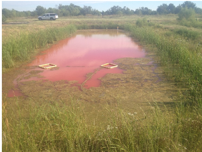
Figure 4.33. RWT flowing through Cell 4N aerator ON (side view).
