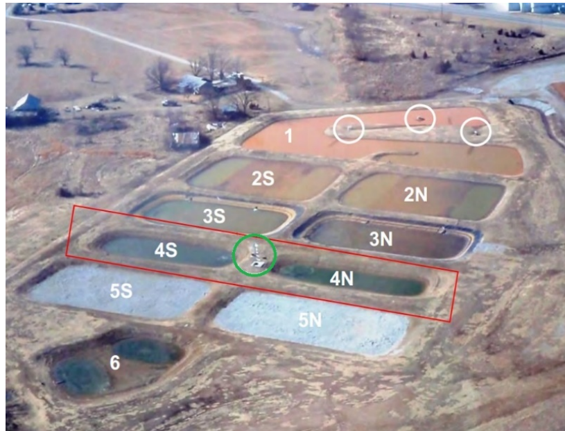
Figure 4.28. MRPTS aerial photo. Cells 4S and 4N in red. The green circle indicate the location of the aeration systems and the arrow points the water flow direction.
