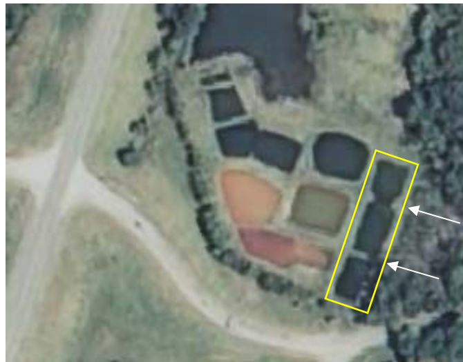
Figure 4.23. Rock Island #7. Cell 3 is outlined in yellow. The white arrows indicated two rock-aeration berms.
