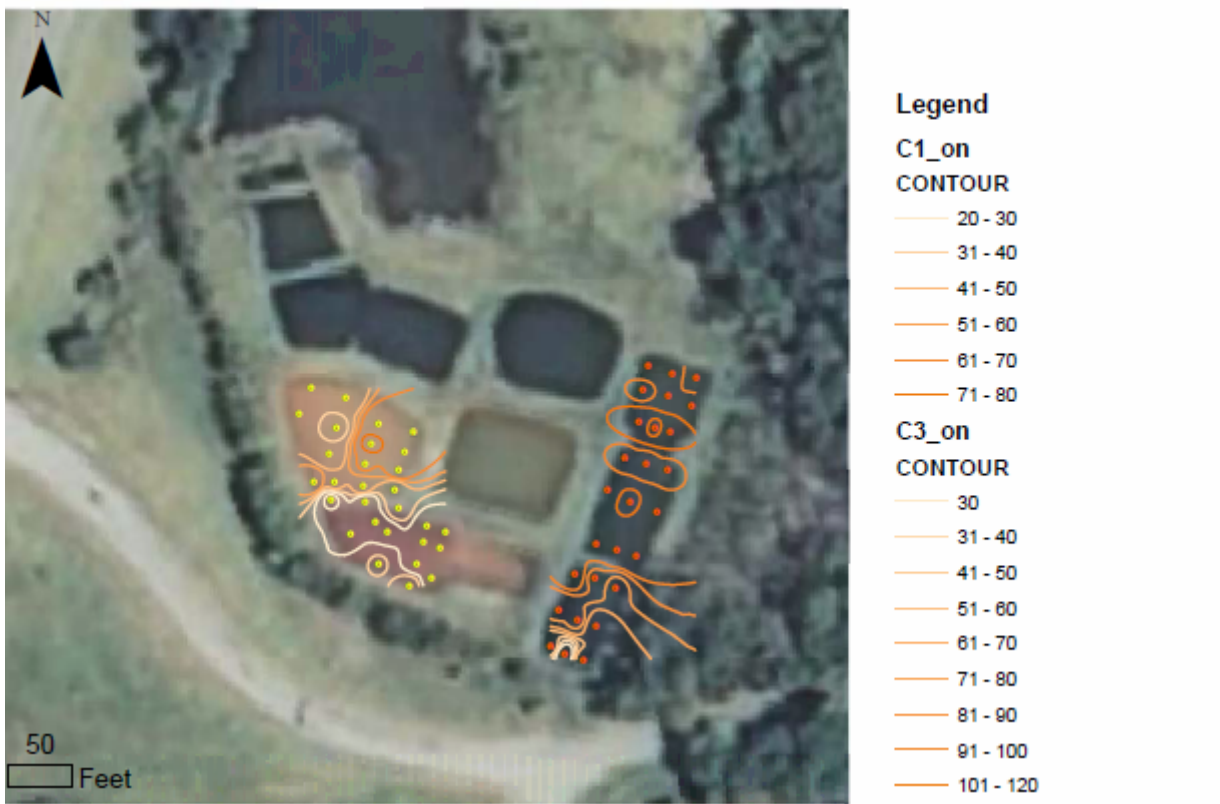
Figure 4.35. Spatial patterns of DO (% saturation) in Cells 1 and 3 at the Rock Island #7 passive treatment system with aerators on.
