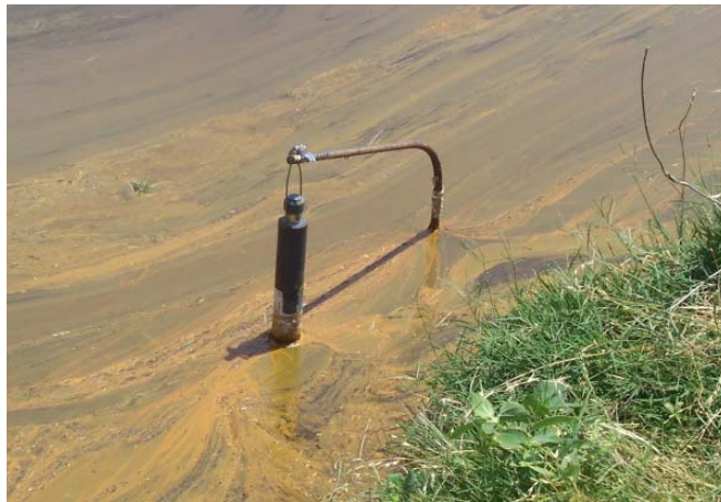
Figure 4.25. YSI OMS suspended above the effluent pipe which is below the water level.
