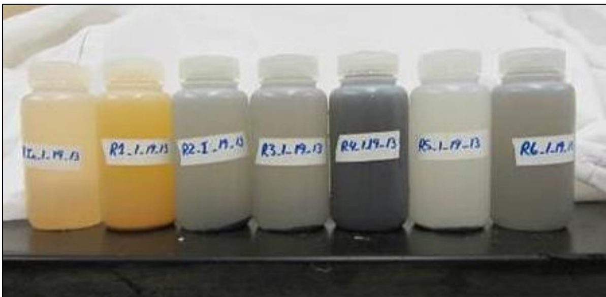
Figure 43: From left to right samples contain influent AMD, limestone only (R1) and bioreactor effluent (R2-R6).
