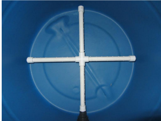
Figure 4: View downward into an assembled reactor displaying perforated “+”-shaped effluent drainage design to allow a spatially equivalent collection of fluid to exit the reactor.
