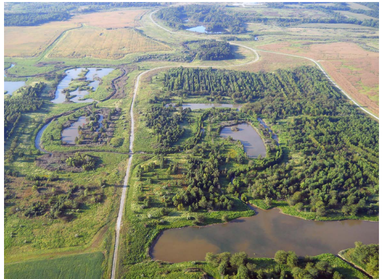
ABOVE PHOTO: A view of the relocated Galum Creek, looking south, taken in July 2011. Several riparian wetlands, in the middle of the photo, were constructed adjacent to the stream. An incline pit is located inline of Galum Creek at the lower right corner of the photo.
