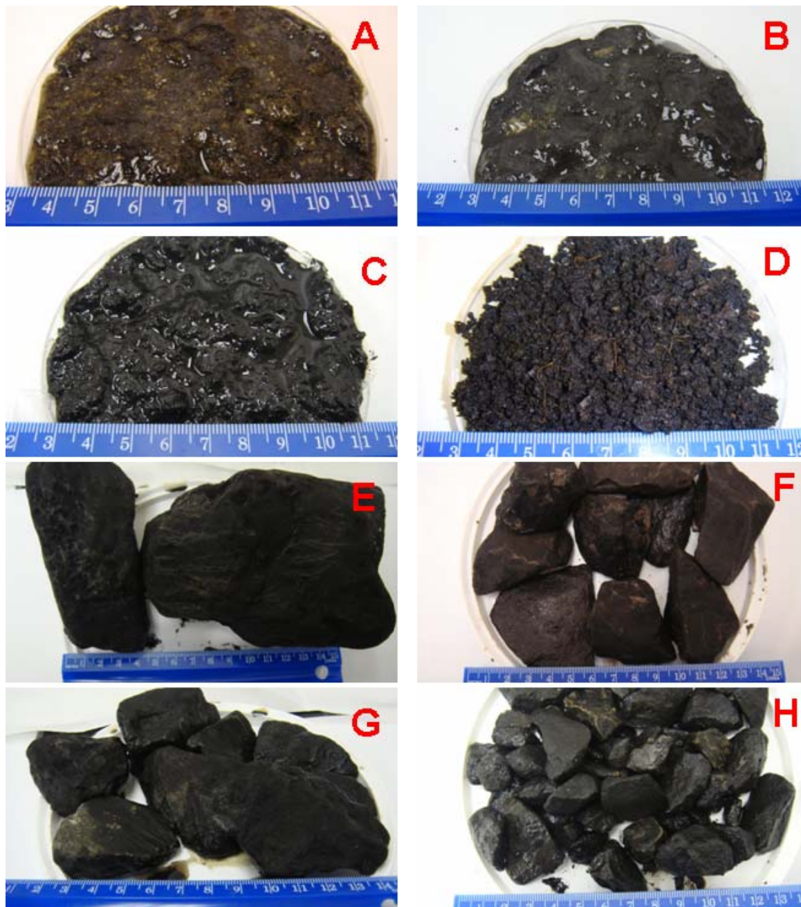
Figure 1. Freshly collected sediments from the Mn(II)-removal beds. A) Ace, B) Glady Fork, C) DeSale 2, D) De Sale 1, E) De Sale 3, F) Fairview, G) Derry Ridge, and H) PBS. Soil-like sediments in A – D. Sediments with MnOx crusts in E – H. Ruler scale = cm.
