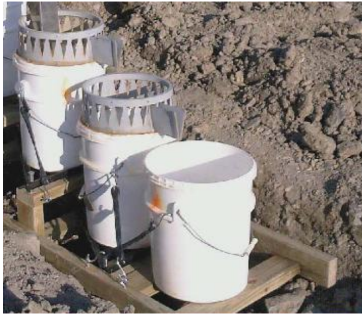
Figure 2-12. Photo showing site arrangement of the divider crown on a bucket.
