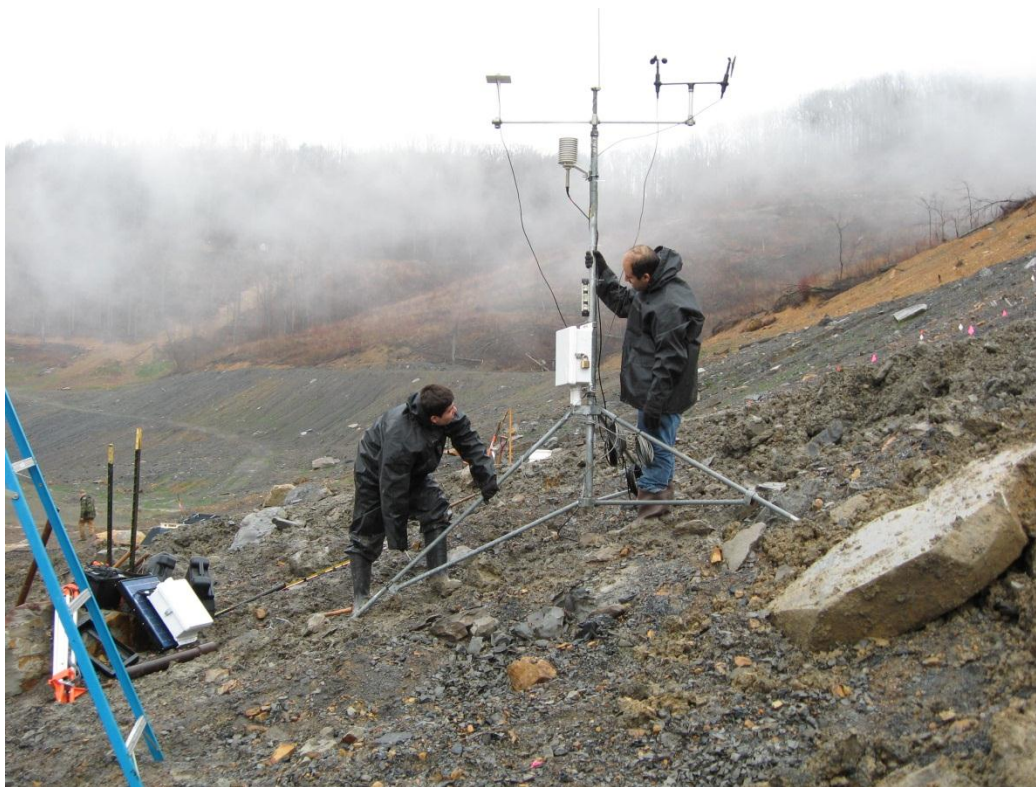
Figure 2-9 Installation of the weather station at Mountainside site.
