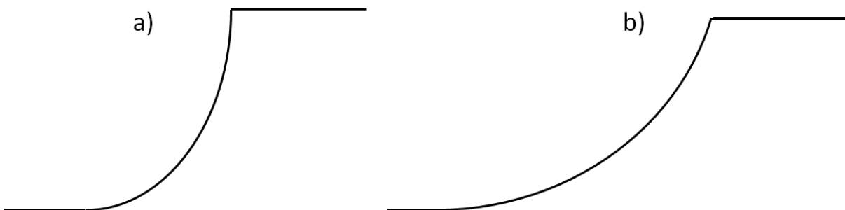
Figure 5-13 Two extreme cases in this conceptual model of slope morphology a) slope in “clayey” material; b) slope in “sandy” material.
