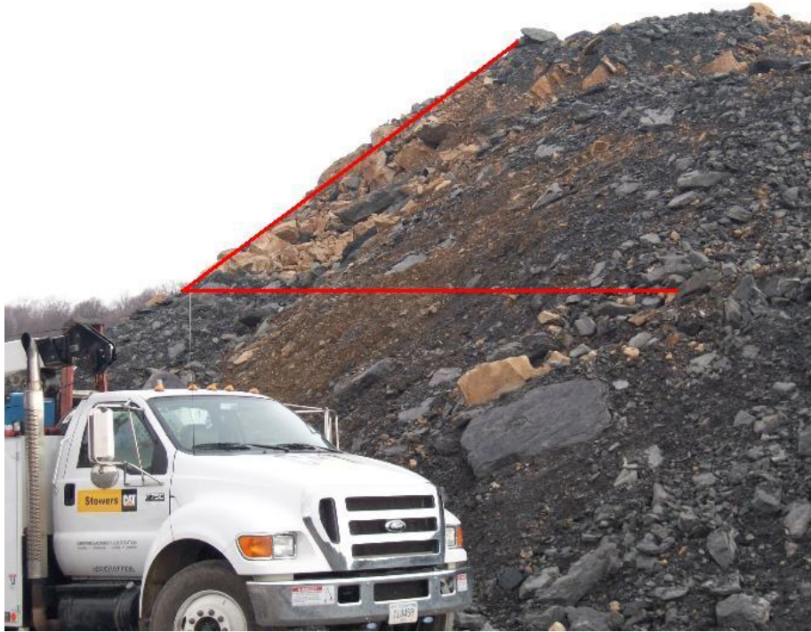
Figure 3-19. Illustration of field determination of the angle of repose at National Site (White 2009)
