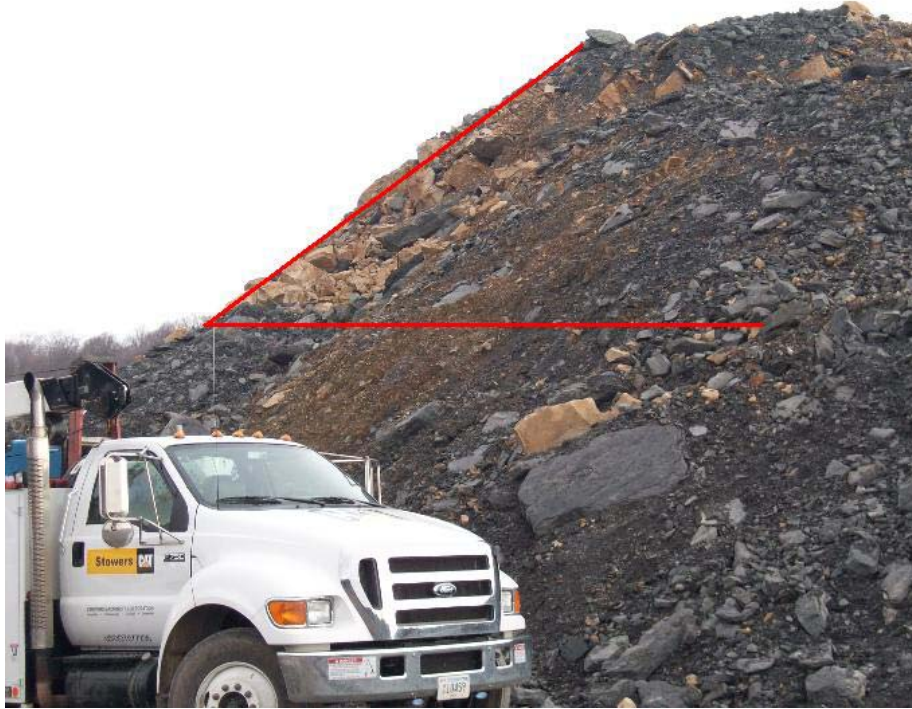
Figure 3-19. Illustration of field determination of the angle of repose at National Site (Aubuchon 2010)
