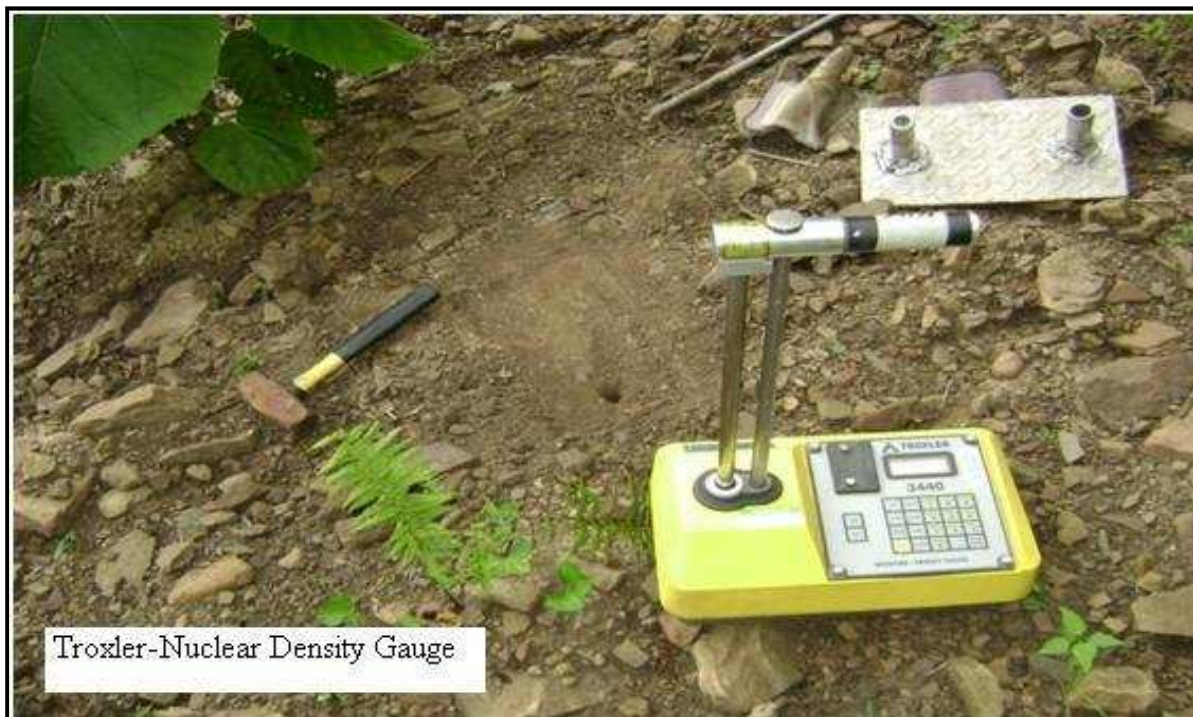
Figure 3.42: Field set up of nuclear density gauge
