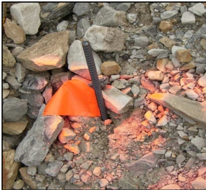
Figure 3.20: A typical survey monument
