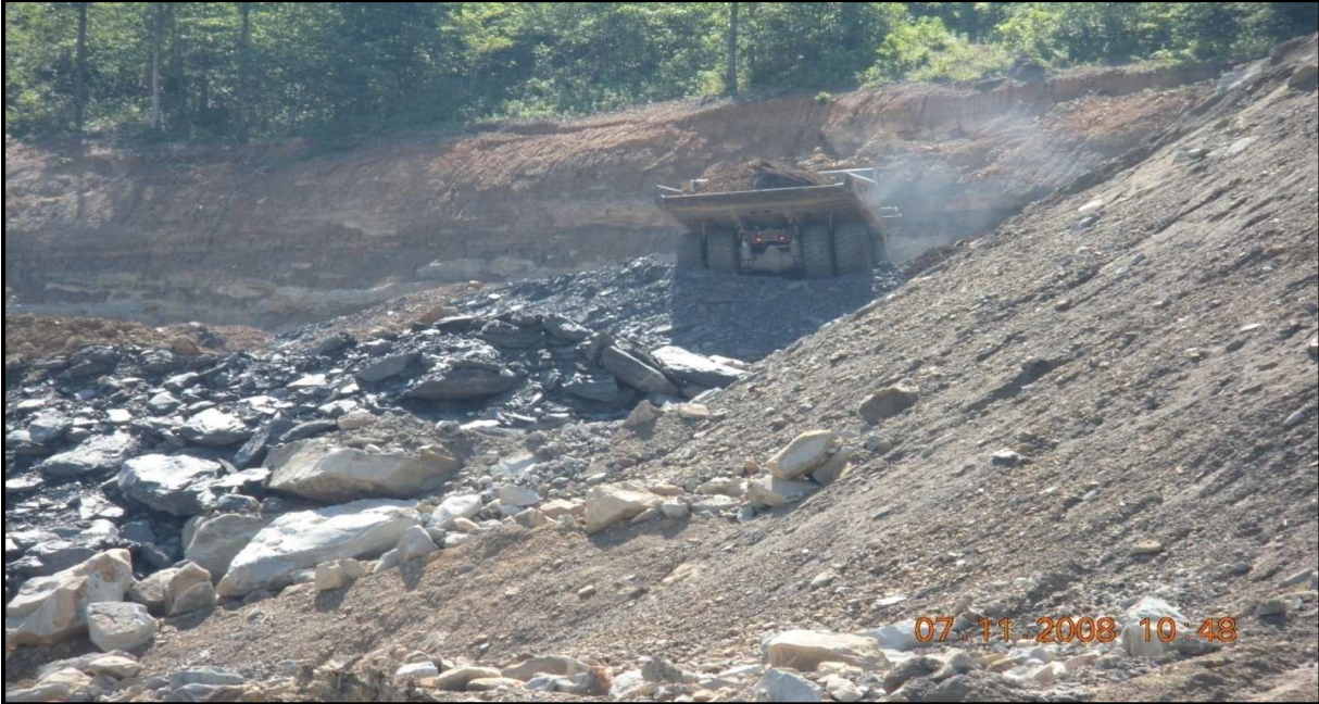
Figure 3.5: Active haulback process (North & South Surface Mine, Logan County, WV)
