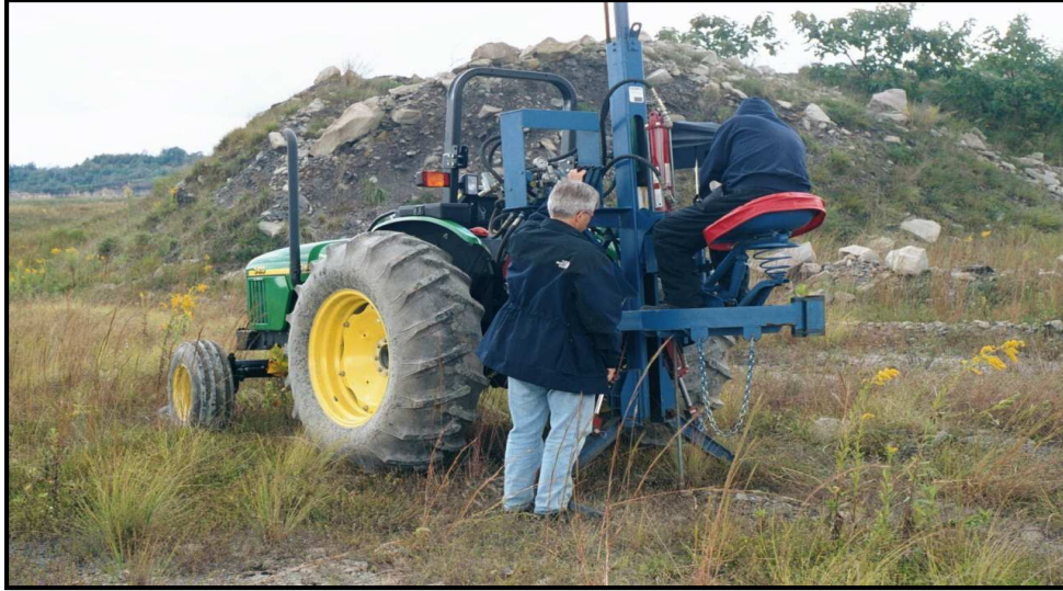
Figure 3.40: Static cone penetrometer used to collect data at the Starfire Mine (Source: Conrad, 2002)
