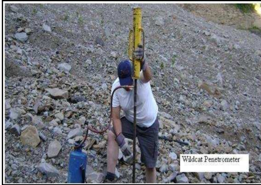
Figure 3.44: Field set up of the Wildcat Dynamic Cone Penetrometer
