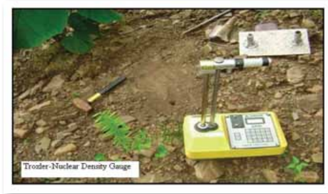
Field setup of nuclear density gauge.
