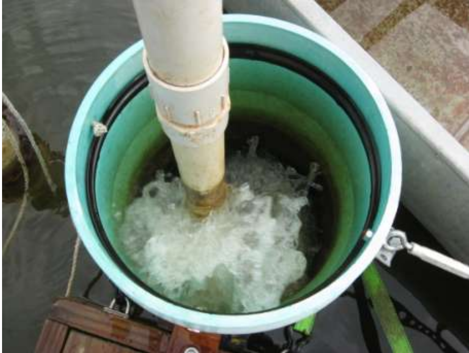
Figure 10. Water production in the 6 inch test pipe.
