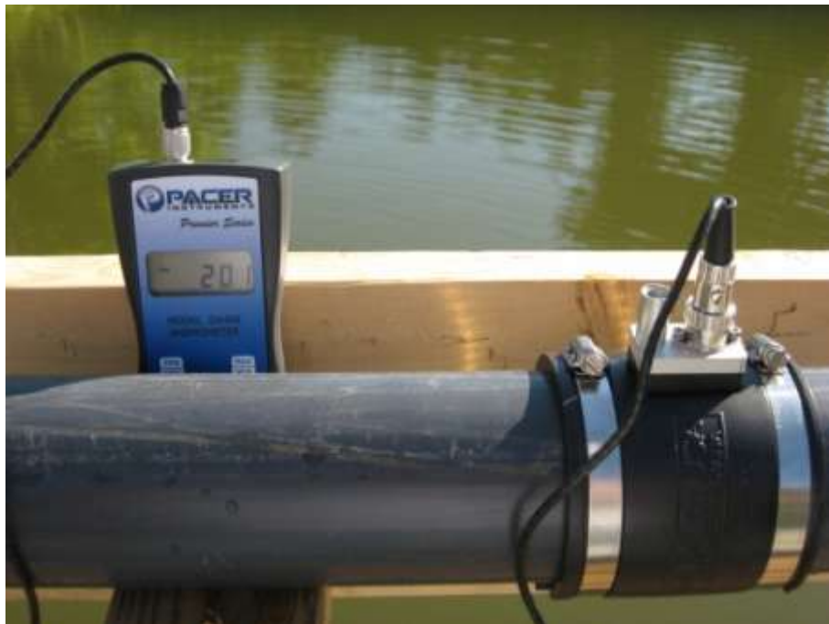
Figure 4. Anemometer in 3 inch SCH 80 PVC pipe
