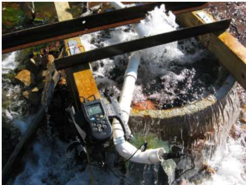
Figure 21. Water produced by the air lift is being measured for pH and DO. (bottom center)
