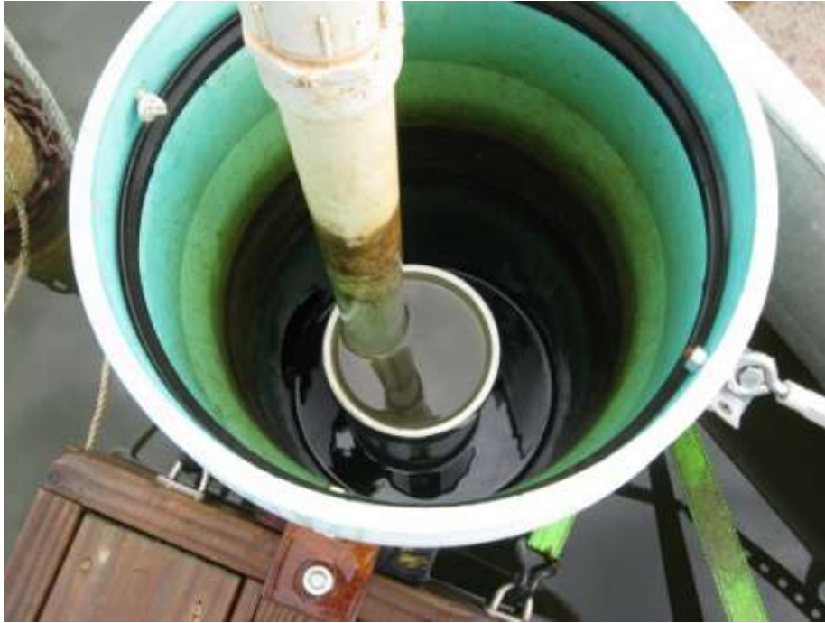
Figure 9. Water level in 6 inch test pipe adjusted to within \frac{1}{4} inch of overflow.
