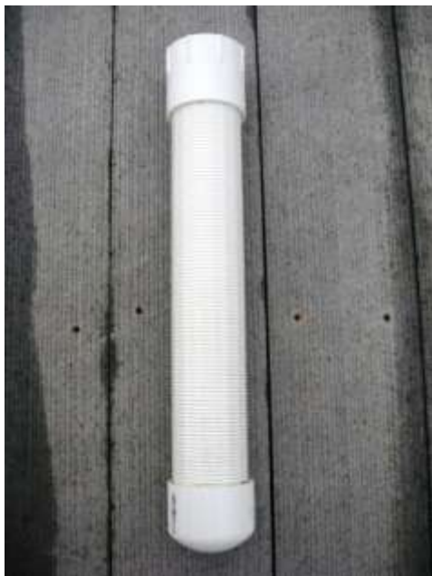
Figure 6. 2 inch continuous slot PVC well screen 0.010 slot, 1 foot exposed screen
