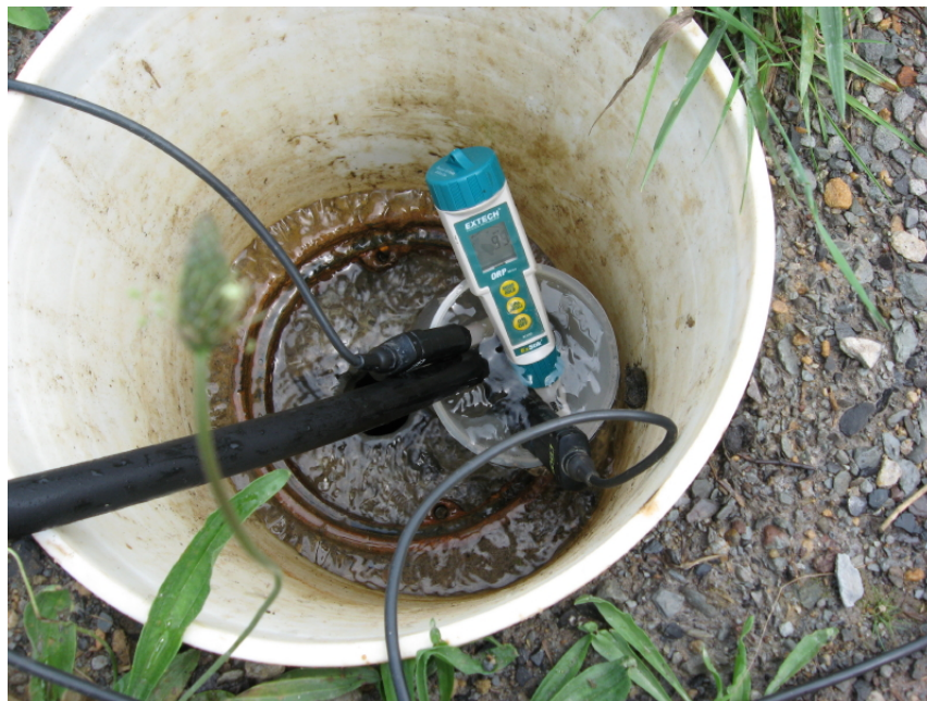
Photo 7. Mine water sampling and injection into the in-by well
