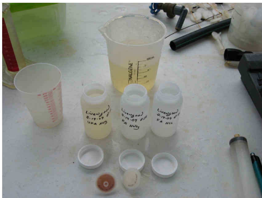
Photo19. Water samples from lt. to rt. unfiltered unacidified; filtered acidified \text{HNO}_3 ; filtered acidified HCl
