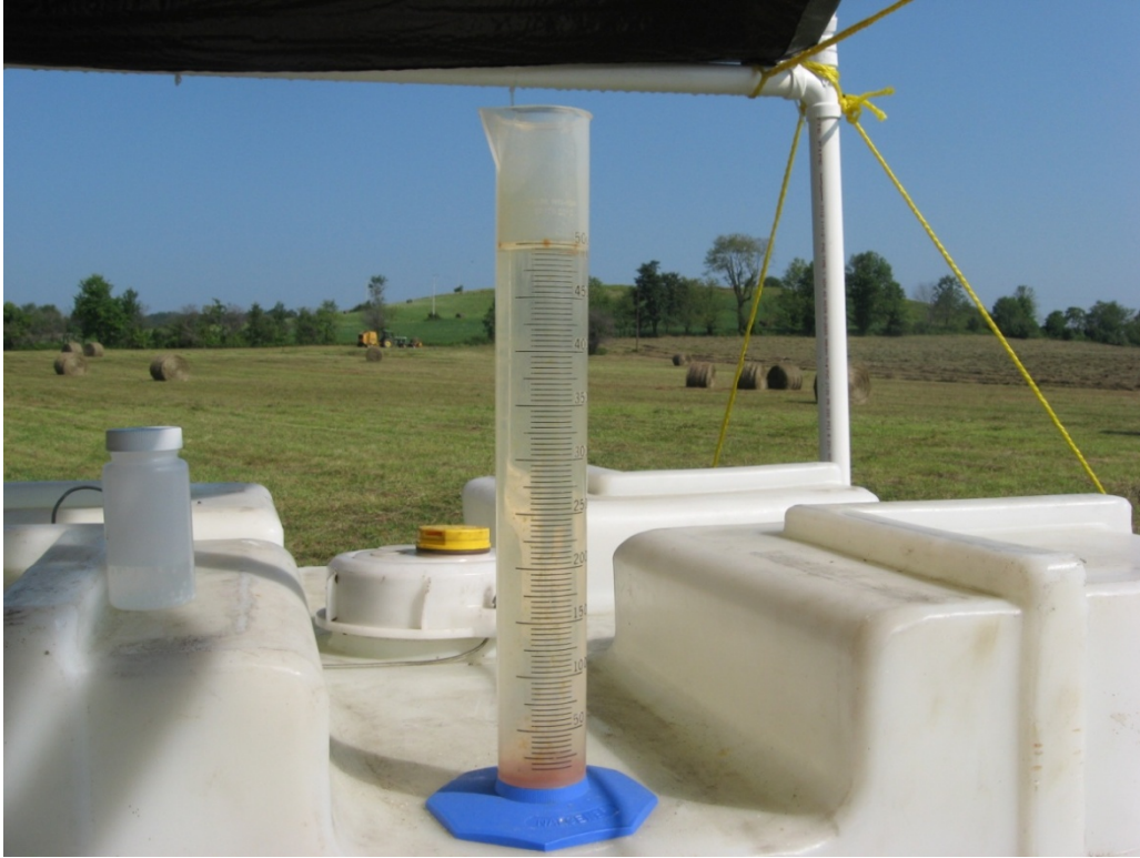
Photo 16. Peroxide treated water after 24 hour settling.
