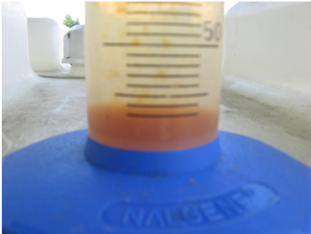
Photo 13. Peroxide treated water 50 minute settling.
