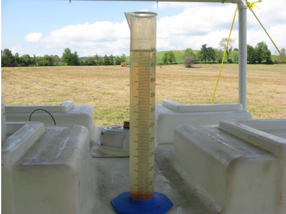
Photo 12. Peroxide treated water 50 minute settling.
