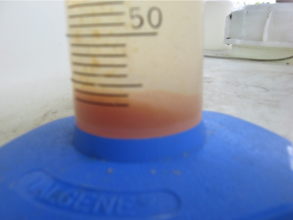
Photo 15. Peroxide treated water 100 minute settling.
