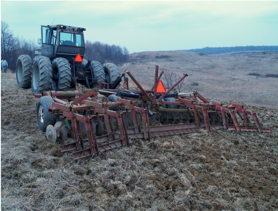
Figure 4. Wjite tractor (240 hp) with plow and disk attachments used to install plots at site.
