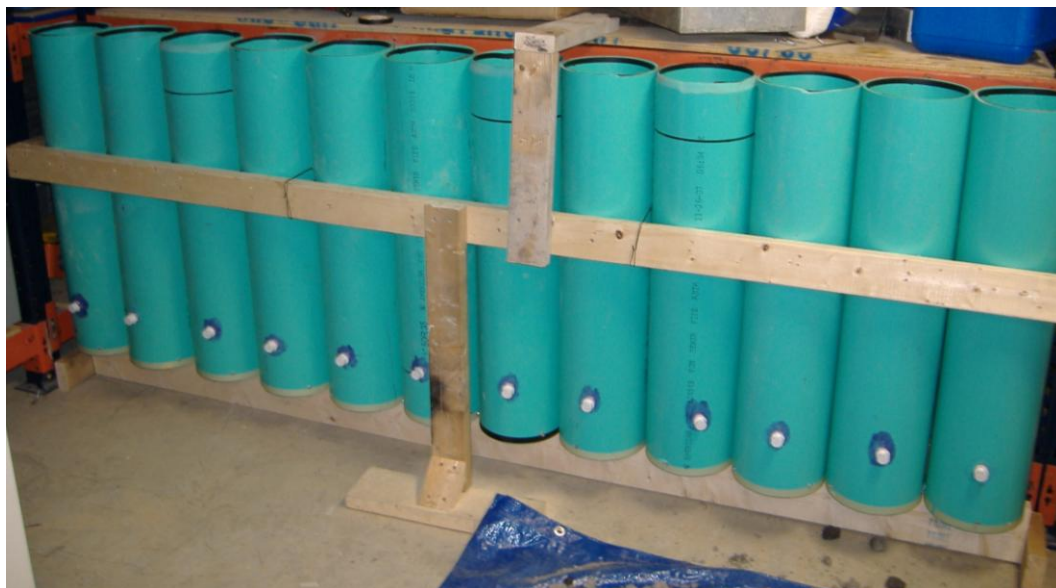
Figure 9. Leaching columns for polymer treatment experiment.
