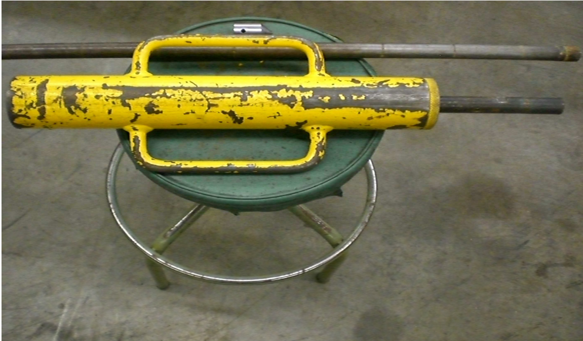
Figure 3.1.3 The Wildcat DCP used to test maximum penetration depth and soil resistance at the Starfire and Gibraltar Mines (shown without the slurry tank).
