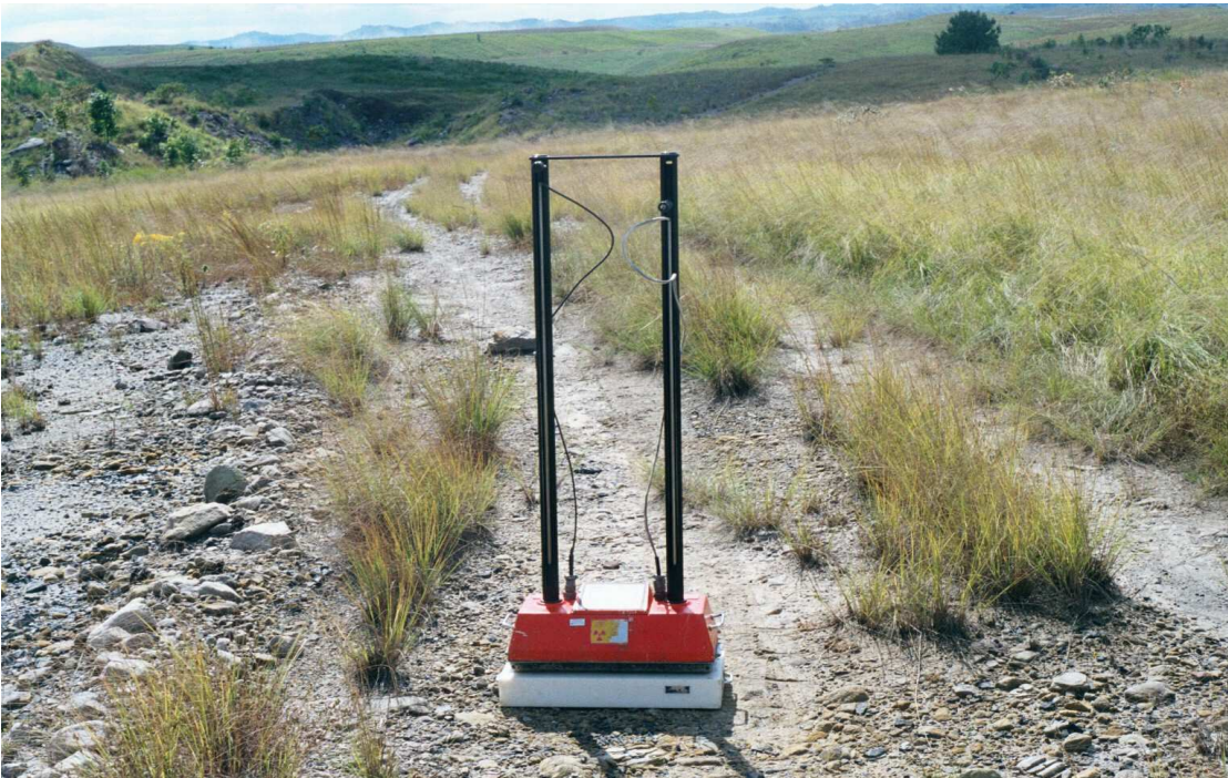
Figure 4.3.1 The Campbell-Pacific Nuclear (CPN) Inc. dual-probe nuclear density gauge used to record density measurements at the Starfire and Gibraltar Mines.
