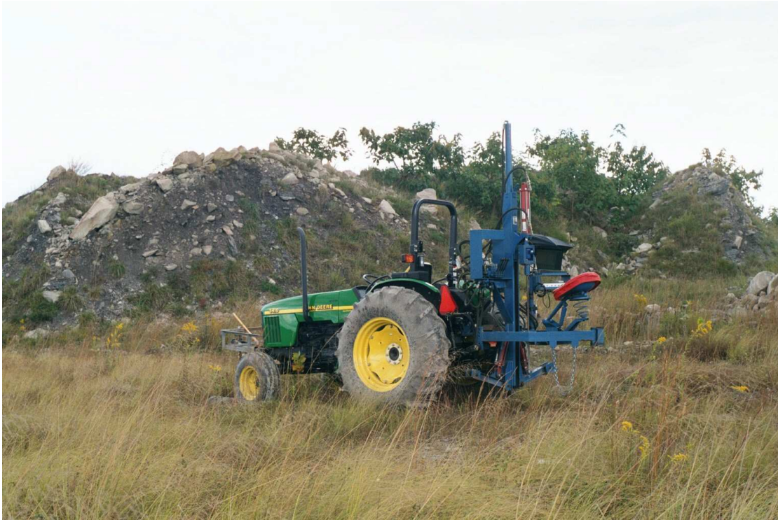
Figure 3.1.2 The workstation mounted on the rear of the tractor for collecting SCP measurements.
