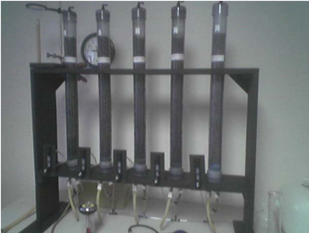
Figure 4.1 Leaching Column Assembly.
