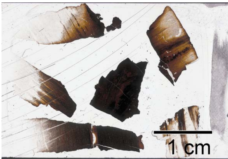
Figure 5.27. Leechburg Coal Refuse (Sample LRBT#2). Scanned image of a polished thin section. The sample is of organic material which complicated sample preparation and resulted in a thin, smeared mount.
