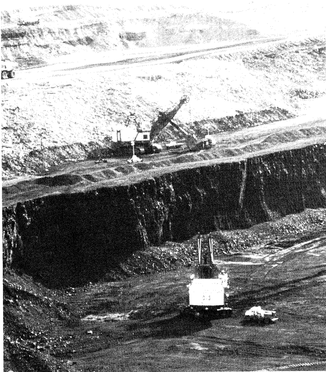
Because of the thickness of the coal seam, open pit mining techniques are used at this western mine.
