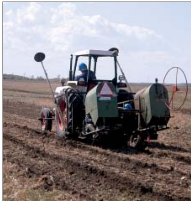
At this reclaimed mine site, tree and shrub seedlings are being planted with a tractor-drawn tree-planting machine. The shelter belts being established will provide field windbreaks and tree and shrub block plantings for wildlife. This woody vegetation creates habitat diversity in the largely open agricultural setting of the North Dakota plains. With over 150,000 trees and shrubs planted at this mine there is more acreage planted after mining and reclamation than existed before. This successful reclamation practice has resulted in an enhanced, long-term agricultural land use.
