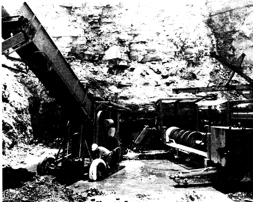
Many eastern mines utilize auger mining to maximize coal recovery.
