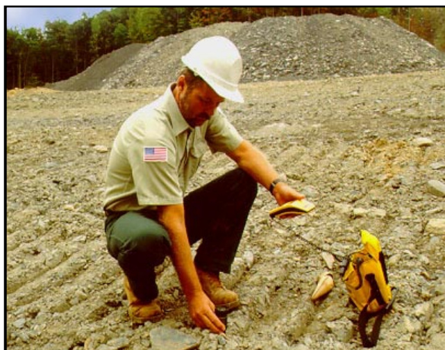
Office of Surface Mining inspector George Olvey checks soil acidity and records the location with a global positioning system receiver.
