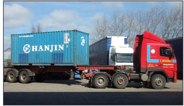
Figure 4.1 Combination Trucks Carrying Intermodal Shipping Containers Boxes with Specially Designed Corners (Can Be Lifted from Above)
