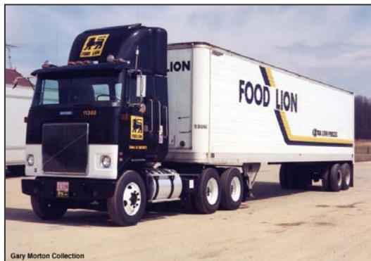
Figure 4.2 Combination and Single-Unit Trucks With “Dry Van” Bodies Similar to Containers, But Connected to Trailers
